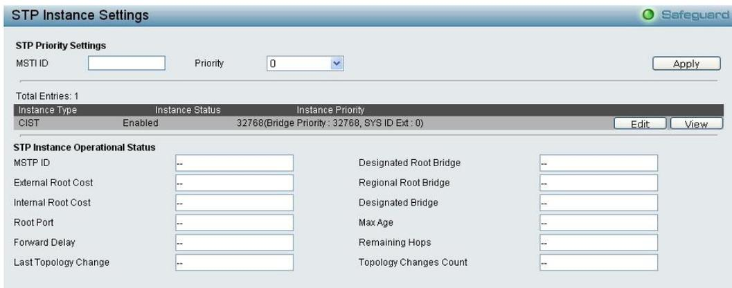
Figure 4.85 - Configuration > Spanning Tree > STP Instance Settings
