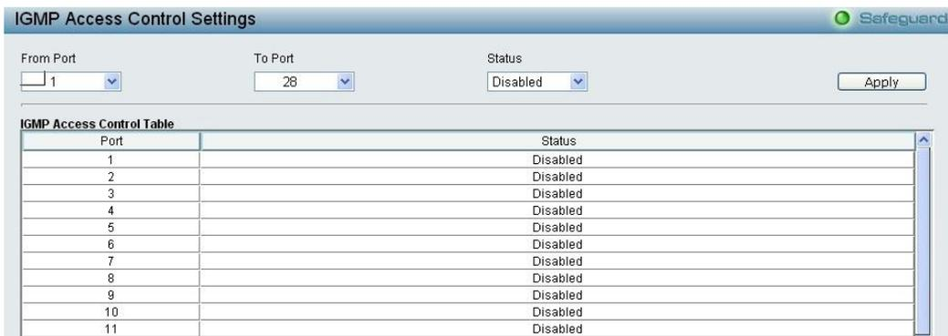
Figure 4.64 – Configuration > IGMP Snooping > IGMP Access Control Settings
