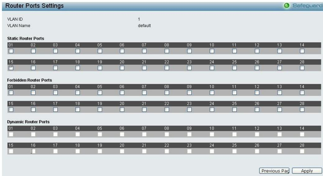
Figure 4.62 – Configuration > IGMP Snooping > IGMP Snooping-Router Port Settings
