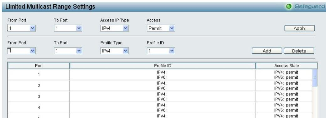
Figure 4.69- Configuration > IGMP Snooping > Limited Multicast Range Settings
