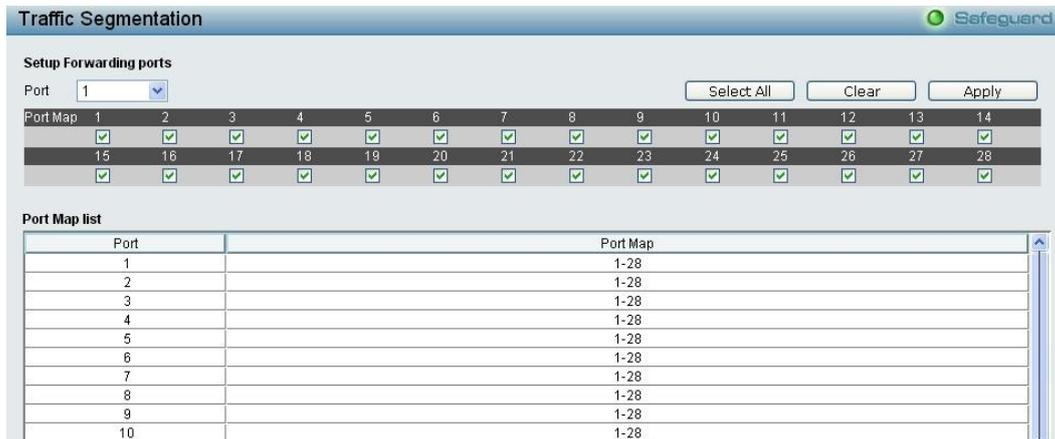
Figure 4.138 – Security > Traffic Segmentation
