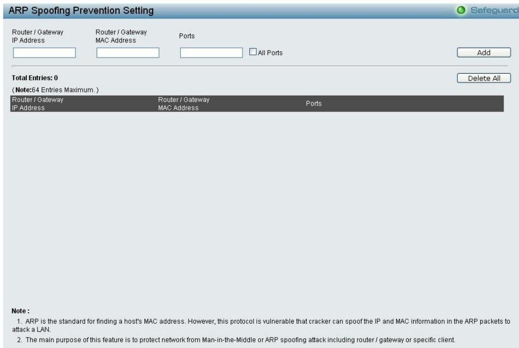
Figure 4.114 – Security > ARP Spoofing Prevention Setting
