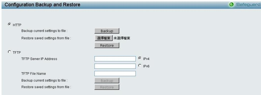
Figure 4.8 – Tool Menu &gt; Configure Backup and Restore
