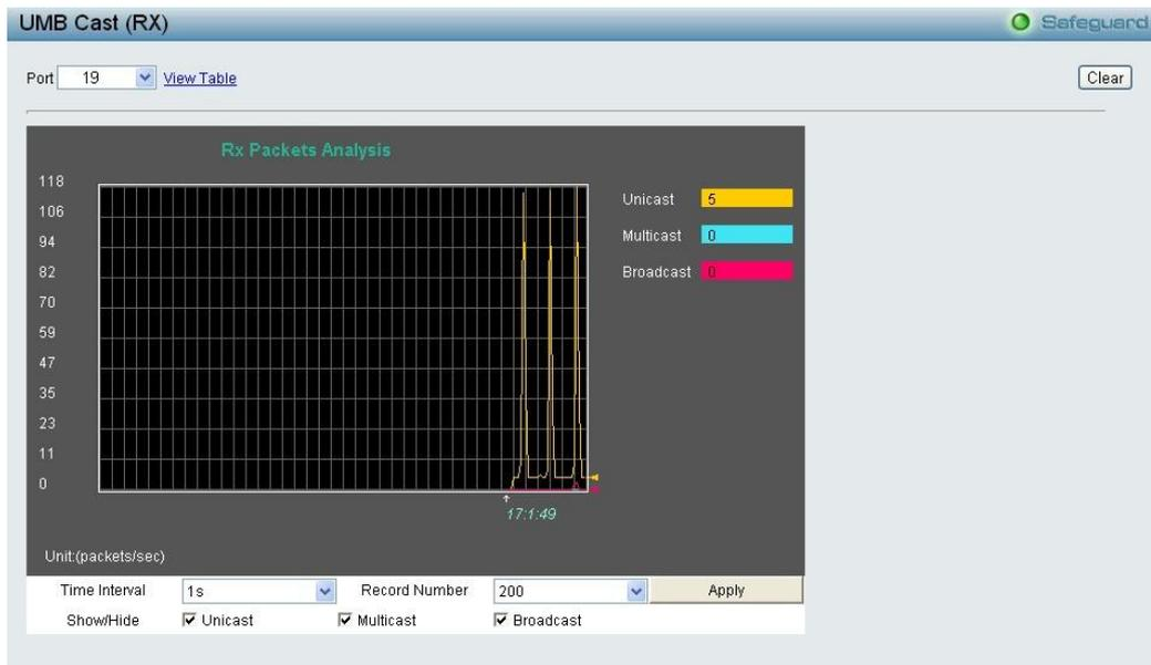
Figure 4.157 - Monitoring > Packets > UMB Cast (RX) (line graph for Unicast, Multicast and Broadcast Packets)
