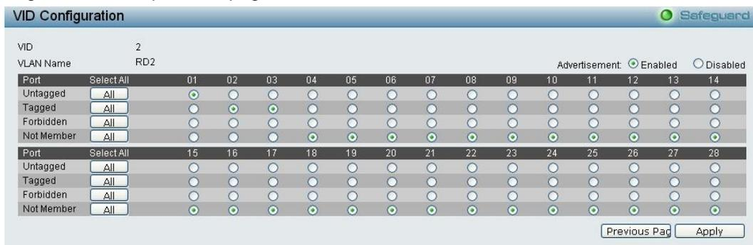
Figure 4.47 - Configuration > 802.1Q VLAN > VID Assignments
