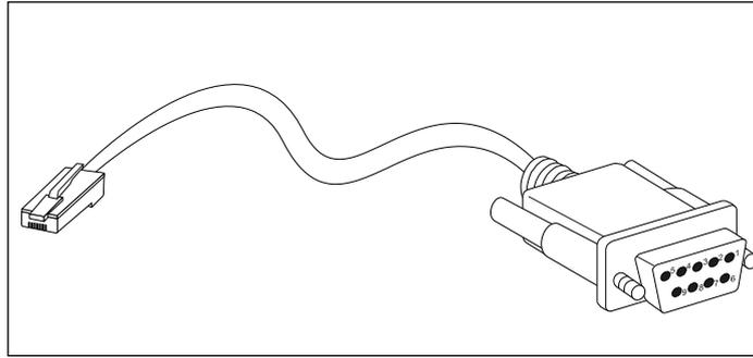
Figure B- 2. Console-to-RJ-45 Cable
