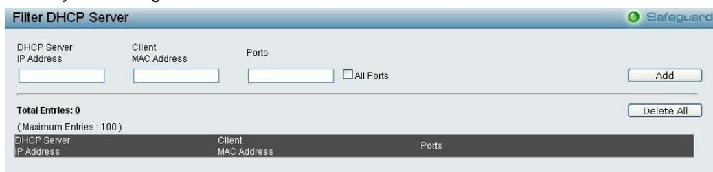
Figure 4.141 – Security > DHCP Server Screening > Filter DHCP Server
