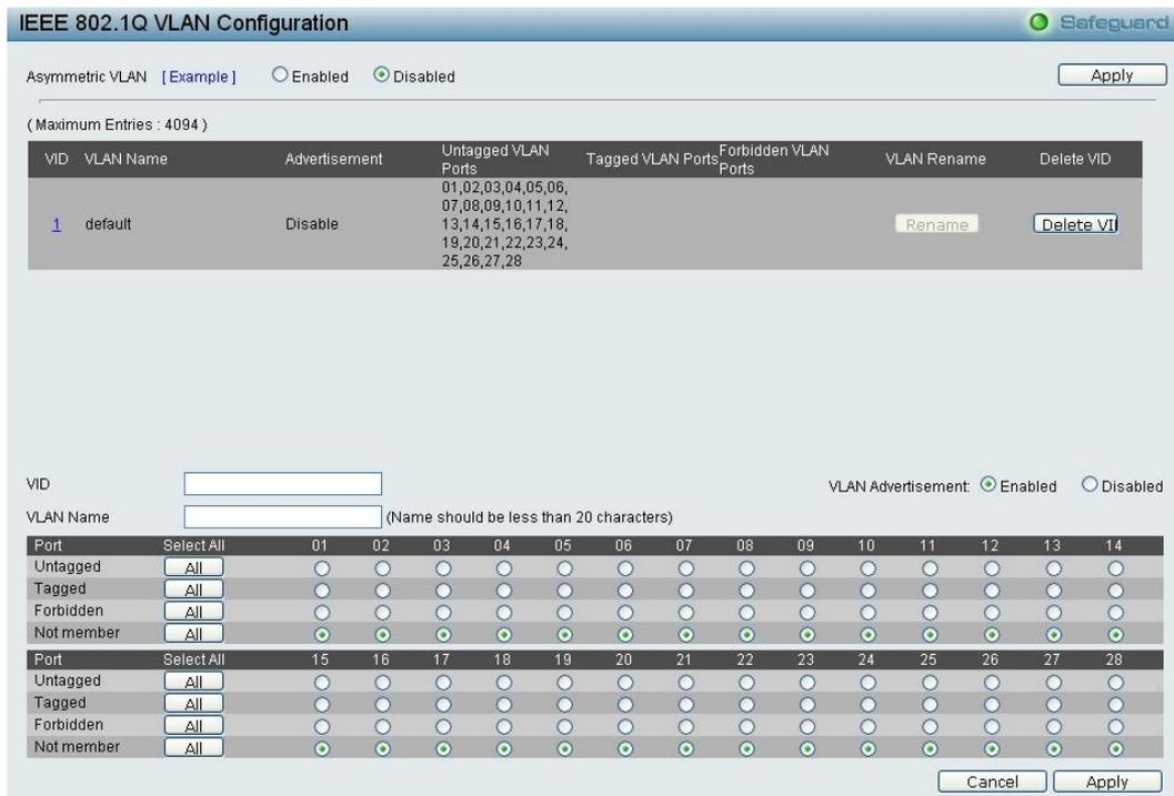
Figure 4.45 – Configuration > 802.1Q VLAN > Add VLAN
